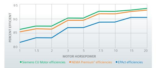
Siemens GP100 motors from 1 to 20 horsepower are available with an optional die cast copper rotor that delivers operating efficiencies above NEMA Premium<sup>®</sup> (NEMA MG1, table 12-12) specifications.
